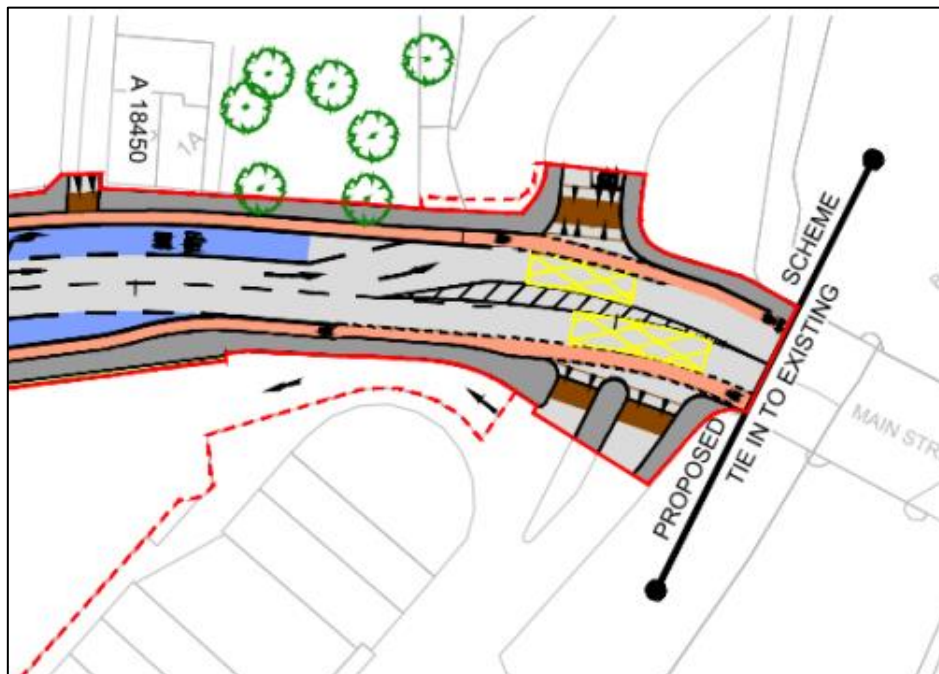
Figure 3.223: Extract from General Arrangement Drawings showing the Proposed Scheme design tie-in to the Existing Design (Sheet 52)
