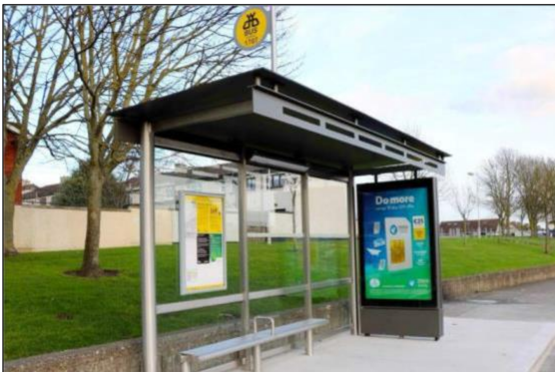
Figure 3.374: Standard 3 Bay Reliance Mark Shelter with Full Width Advertising Panel (Source: PDG)
