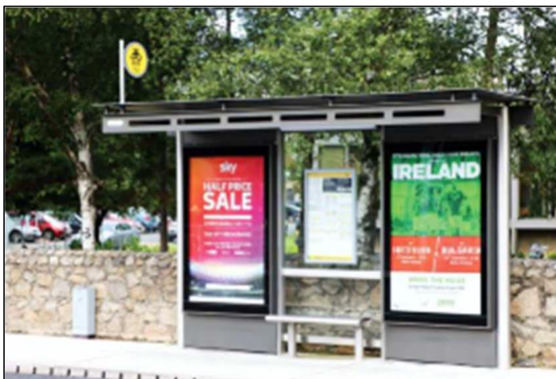
Figure 3.376: Example of a 3-Bay Reliance Cantilever Shelter with a Narrow Roof Configuration With and Without Half End Panels (Source: PDG)
